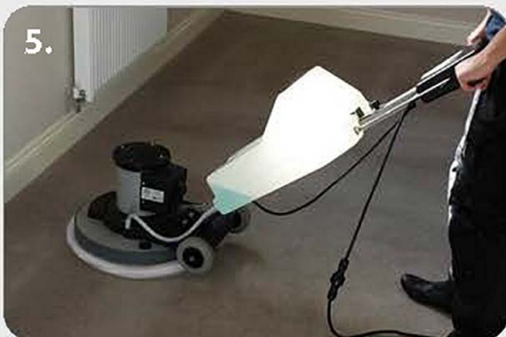
5. Bonnet Absorption - Absorb and warm carpet fibres to remove as much excess moisture as possible to speed drying.
